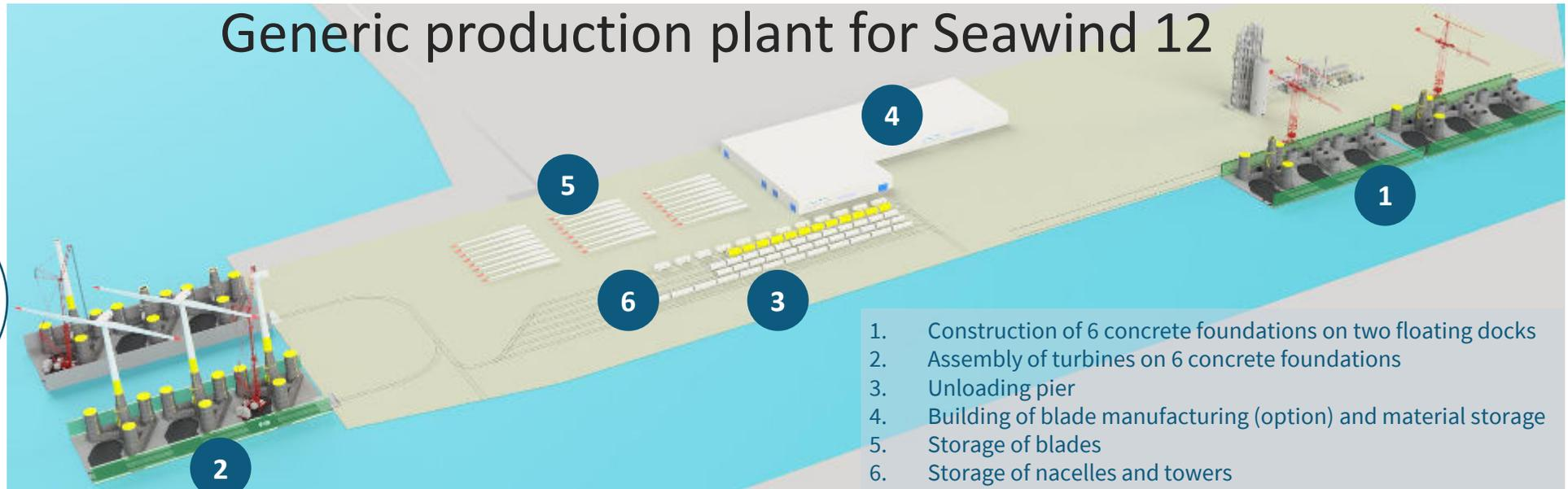
1. Construction of 6 concrete foundations on two floating docks
